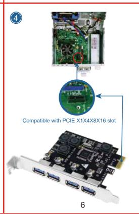
**Step3**,Reattach the computer cover,and put back 2.Find this added on USB card hardwae in Windows system "Device Manager" and check if system read it. removed peripherals, power on desktop computer.
